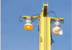
Crane boom light after collision
